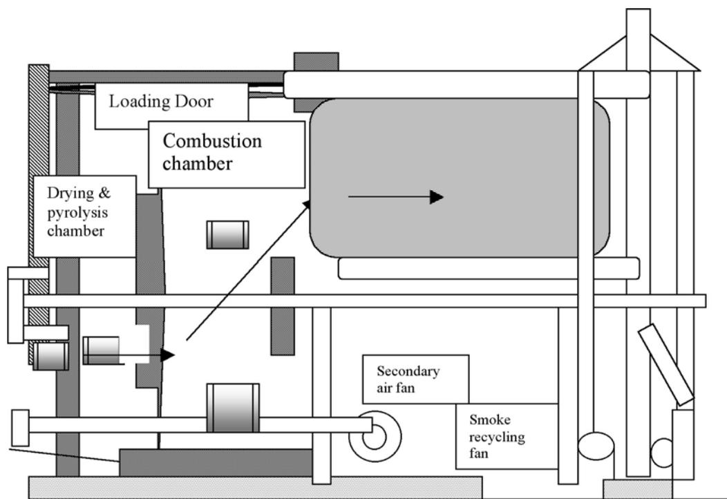
Figure 3. Sectional view of the pre-combustion chamber for bunch stalks.
