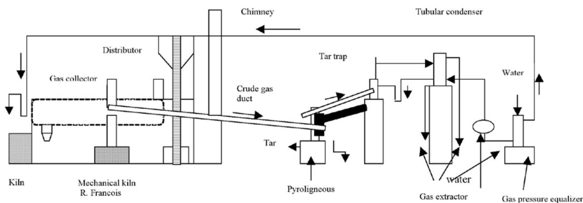
Figure 4. Schematic layout of a carbonization installation.
