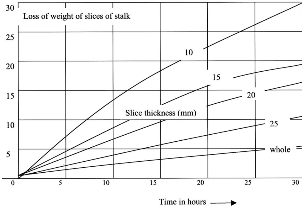
Figure 2. Desiccation curves of bunches stalk in relation to slice thickness and time of desiccation.
