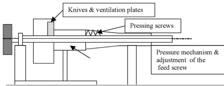
*Figure 1. Bunch stalk shredder.*
