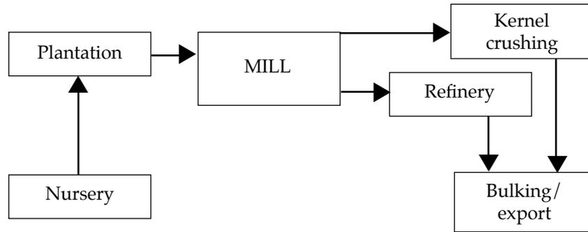
Figure 1. Flow diagram of the palm oil industry.
