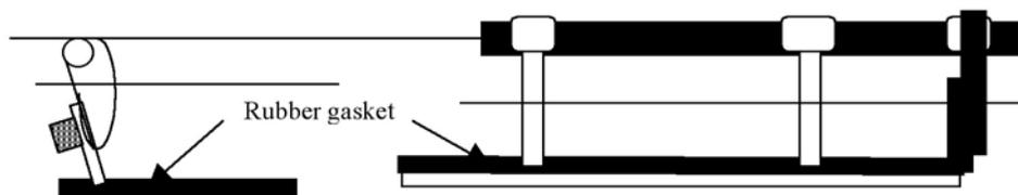
Figure 1b. Detail of removable baffles.
