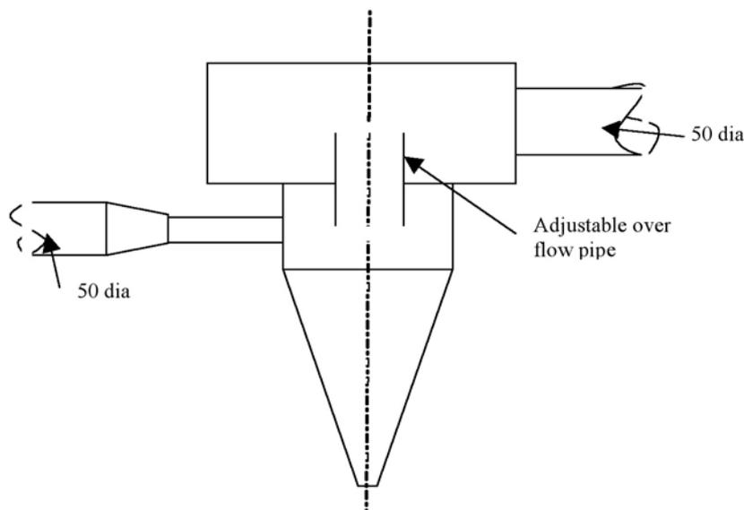
Figure 2. Sand cyclone capacity 12.5 t hr<sup>-1</sup>.
