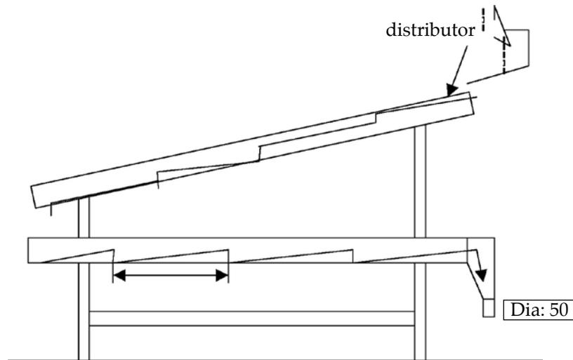
Figure 1a. Step desanding installation – width 70 mm capacity 2 t hr<sup>-1</sup>.
