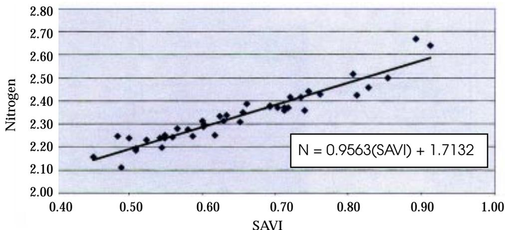
Figure 4. Foliar nitrogen versus SAVI with linear fit line.
