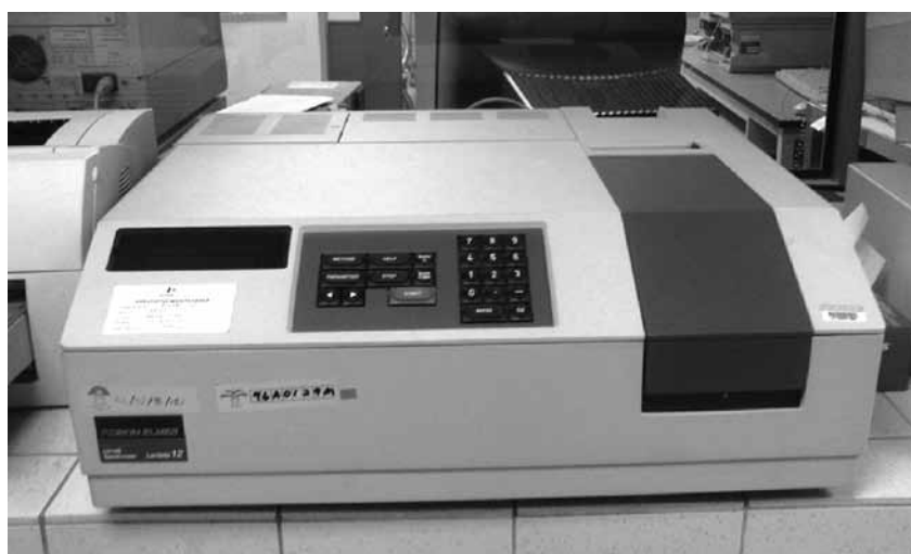
Figure 1. Perkin Elmer Lambda 12 UV-VIS Spectrometer (for sample analysis).
