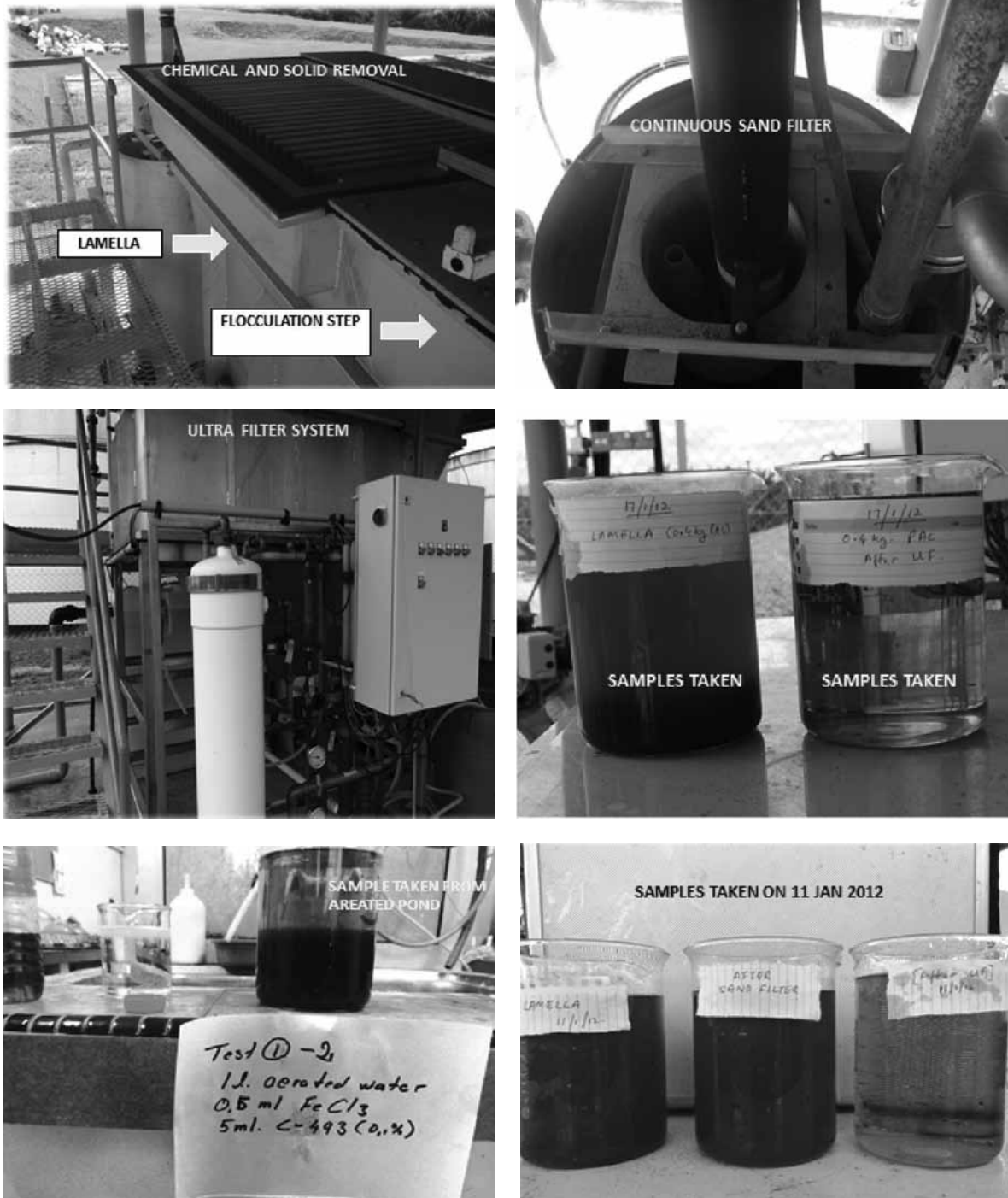
Figure 3. Stages of waste water treatment (BCMM) system.
