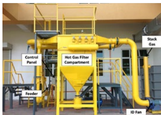
Figure 6. Pilot plant of hot gas filtration system.
