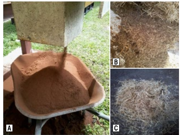
Figure 4. Products from the NTS plant, (A) PKS powder, (B) EFB, and (C) OPF.
