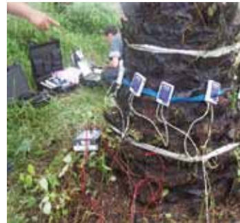
Figure 1. Installation of sound sensors on the oil palm stem for the detection of Ganoderma infection.
